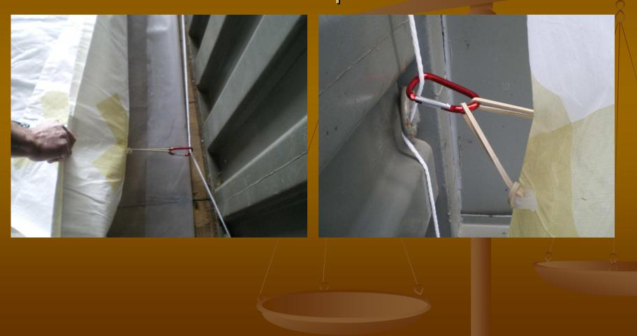
Secure all the ceiling and floor ties to the suspension rope until you reach the container doors. At this point if possible secure the clip to the lash ring or channel bar.
