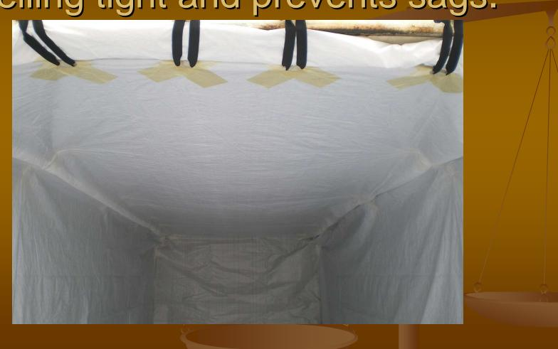
The liner is now ready to load. Once loading is complete, gather the end together, twist and cable tie the opening closed.
