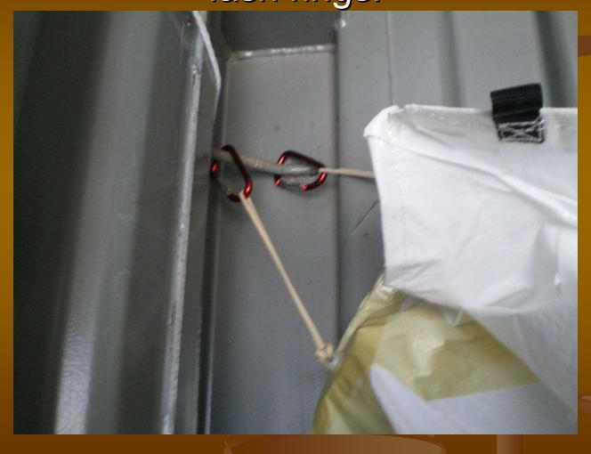
Locate the next set of clips moving toward the rear of the liner and secure to the suspension rope.
