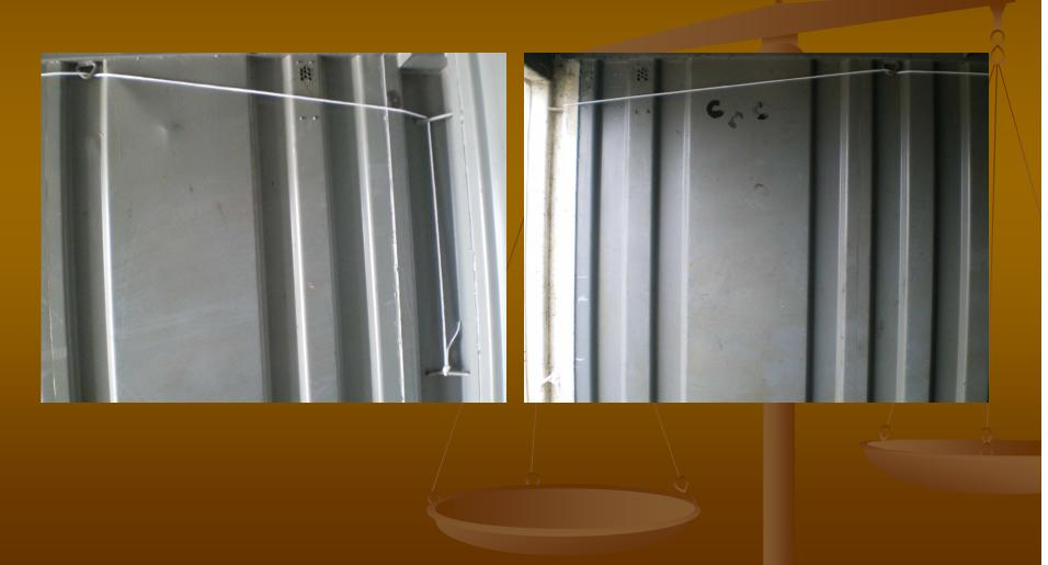
Next feed a rope through the floor container lash rings and tie to each corner or the last lash ring.
